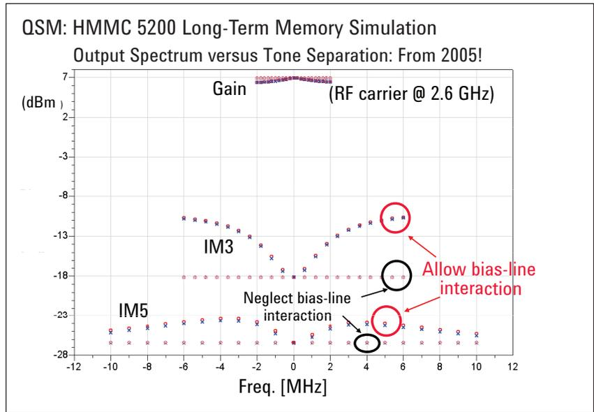
Figure 2. When bias-line interaction is allowed, the offset frequency dependence and the absolute value of the distortion (as measured by IM3) can change dramatically.
