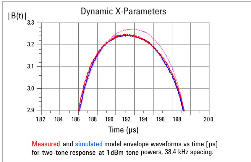
Figure 5. Measured (red) and simulated (blue) dynamic X-parameter model envelope waveforms versus time for a two-tone response of an amplifier. The magenta waveform is the result of using a one-tone static X-parameter model.
