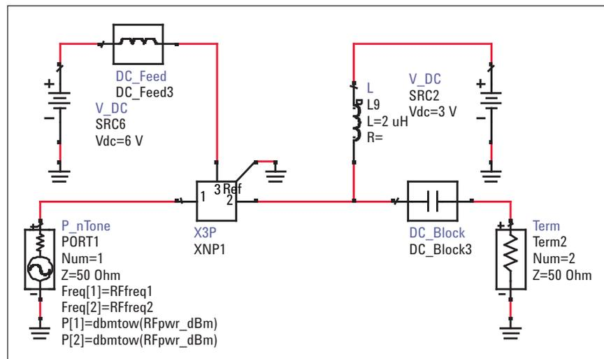
Figure 1. An X-parameter model, extracted under true static bias conditions, can be used to model a component's quasi-static memory effects with respect to bias modulation.
