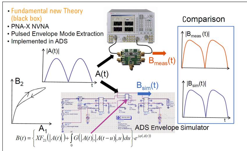
Figure 4. Dynamic X-parameters extends the application of X-parameters to memory effects beyond the quasi steady state.
