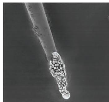
Figure 3. Low voltage image of uncoated electrode with CNTs on tip.
