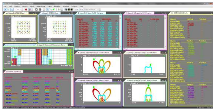
Figure 7. 8-channel TD-LTE beamforming with antenna patterns and EVM measurements per layer. The same measurement is available for LTE-FDD.
