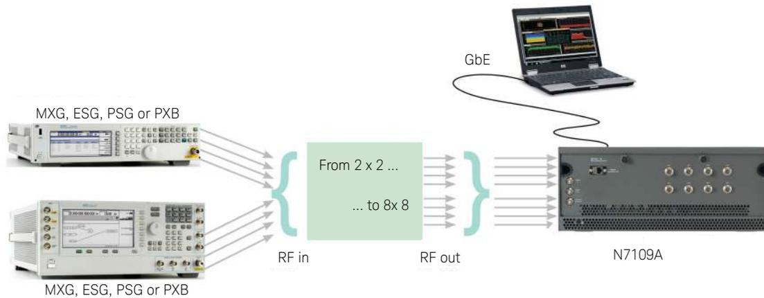
Figure 1. Typical MIMO test setup.
