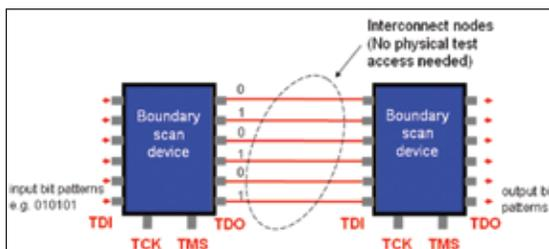
**FIGURE 1.** A simple chain of boundary scan ICs.
