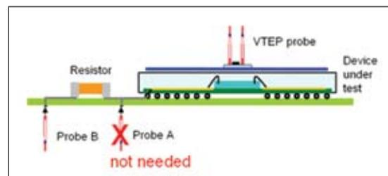
**FIGURE 2.** DriveThru injects a stimulus signal through a passive component directed toward the DUT.
