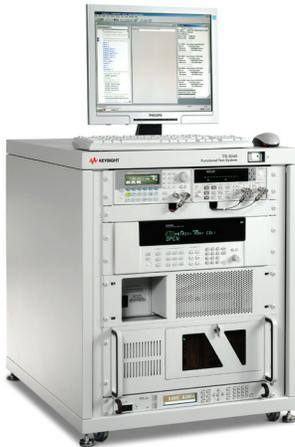
TS-5000 systems can include, as standard, a 320 x 4 line signal switching matrix, load switching up to 30 amps, multiple power sources up to 1200 W, a DMM, counter and a function/arbitrary waveform generator. To extend this configuration you can specify additional test resources from Keysight's wide range of standalone, modular, and card-cage instrumentation in order to create a system that meets your exact functional test needs.
