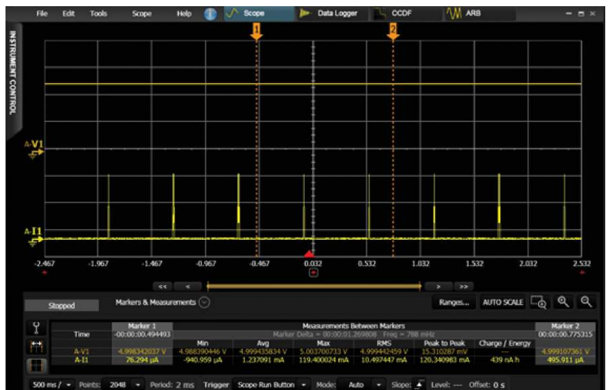
Figure 5: Scope acquisition with markers
