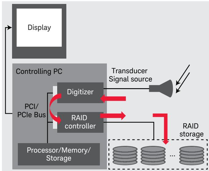
Figure 4. Recording to a RAID array can provide tremendous capacity when large volumes of data must be acquired.
