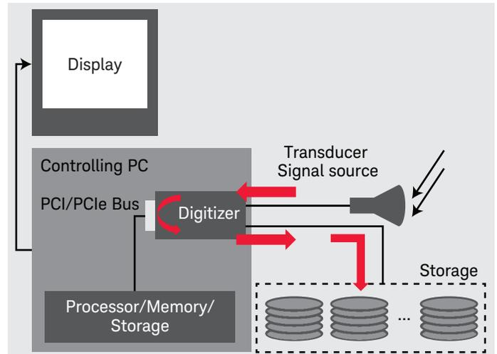
Figure 3. Recording directly to an external disk drive provides maximum performance in streaming applications.
