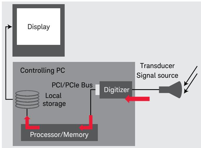
Figure 2. Recording to the host processor is the simplest approach, even if multiple digitizers are required.
