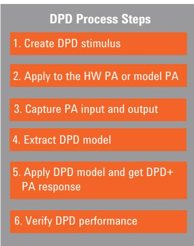
FIGURE 3. Using the setup in Figure 2, the DPD modeling flow is a 6-step process
