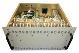
port chassis, which then connects to the vector network analyzer. The matrices are constructed from low-loss, single pole, six-throw electromechanical switches and are designed for expansion, up to a total of 216 ports. The test head is attached to the DUT with screw-on connections and matched semi-rigid cables in order to minimize signal losses.
