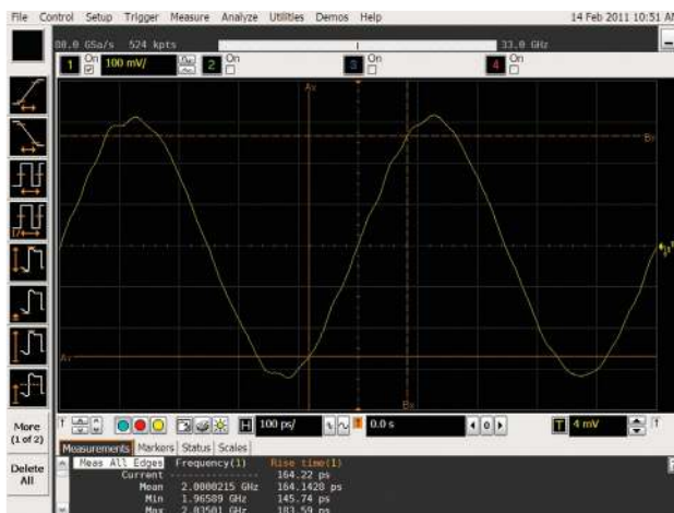
Figure 2. When the sine-wave frequency decreases, the time-interval error increases.
