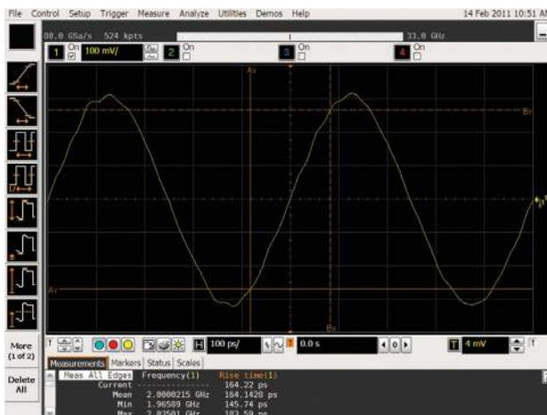
**Figure 2.** When the sine-wave frequency decreases, the time-interval error increases.
