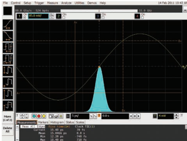
Figure 6. The oscilloscope's noise contribution to jitter measurement increases as rise times increase, as shown for this 90000 X-Series scope.
