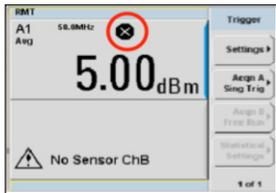
Figure 2. Triggering mode in Single Trigger
