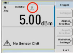
Figure 1. Triggering mode in Free Run
