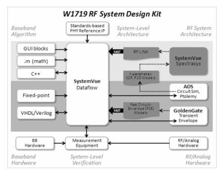
Figure 2. The W1719 RF System Design Kit is an optional add-on to SystemVue that enables deeper insights and RF design flow connectivity than would be possible using only a dataflow simulator.
