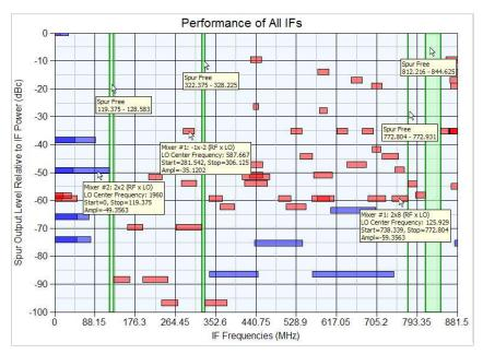
Figure 4. The WhatIF frequency planning tool quickly shows the best choices of IF frequencies for best spur-free performance and with lower system complexity.
