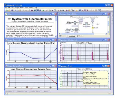
Figure 3. Spectrasys accounts for complex mismatch, bi-directional propagation, nonlinearities, frequency response, leakage terms, continuous spectrums from DC to millimeter waves, and tracks individual signal and noise contributors. These can be inspected interactively in seconds, directly from the graphs.
