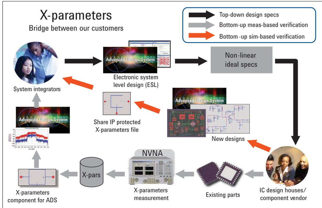
Figure 2. X-parameters can be created from measurement or ADS simulation with the same speed and convenience as the well-known linear S-parameters.
