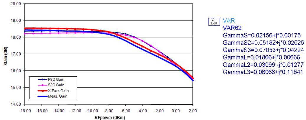
Figure 4. A comparison of the simulated and measured gain compression results, with the frequency at 715 MHz. The source and load reflection coefficients up to the 3rd harmonics are given.
