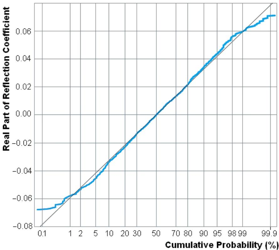
Figure 12. Normal probability plot of spectrum analyzer input reflection, 0 to 3.6 GHz, 10 dB attenuation.
