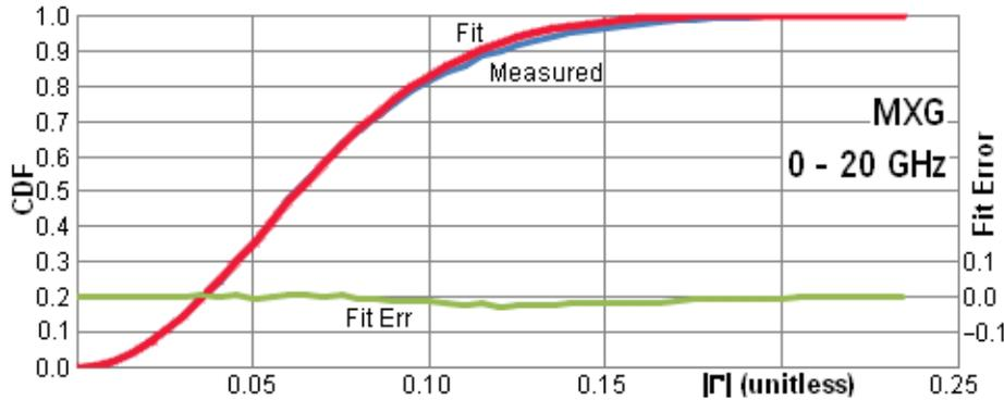
Figure 10. Cumulative distribution functions for N5183 signal source, 0 to 20 GHz.
