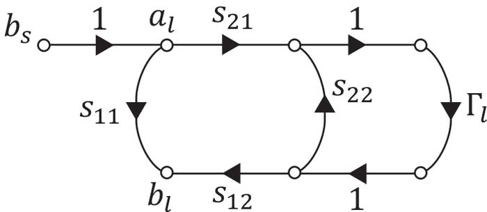
Figure 5. Single discontinuity as a two-port element.
