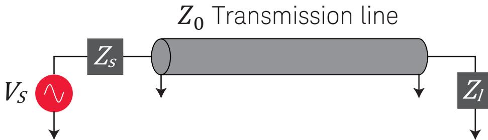
Figure 1. A generator connected to a load through a transmission line.
