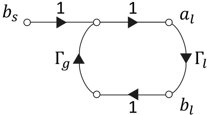
Figure 3. Simplified circuit model.
