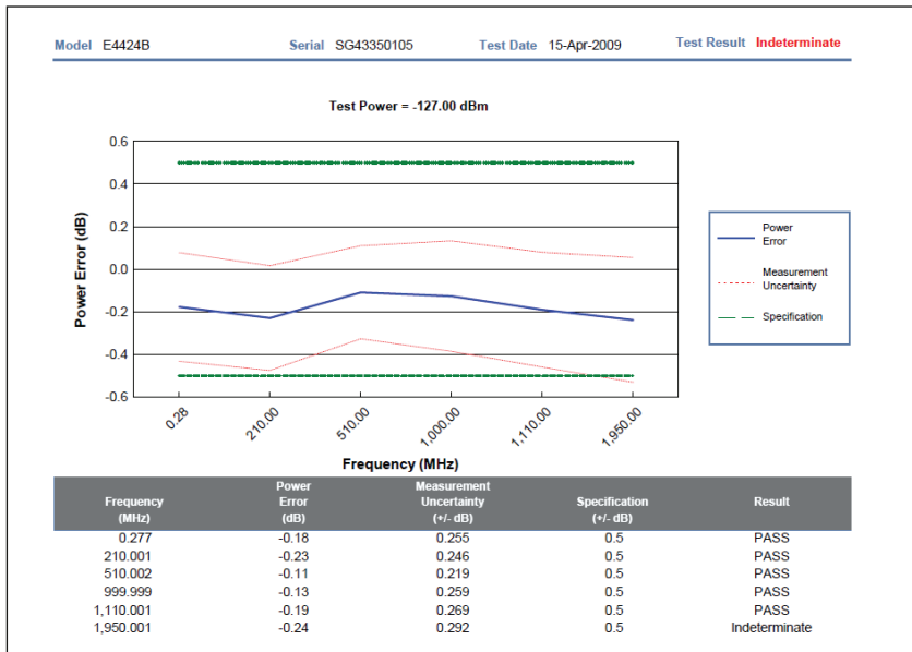
Figure 4. Offset or bias results in reduced margin at the highest frequency.
