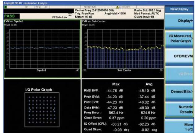
Figure 2. "OFDM EVM" displays four traces with EVM vs. symbol, EVM vs. subcarrier, constellation, and measurement results.
