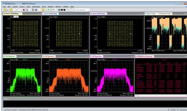
Figure 2. 3-channel 802.11ac analysis using Keysight's 89600 VSA software.
