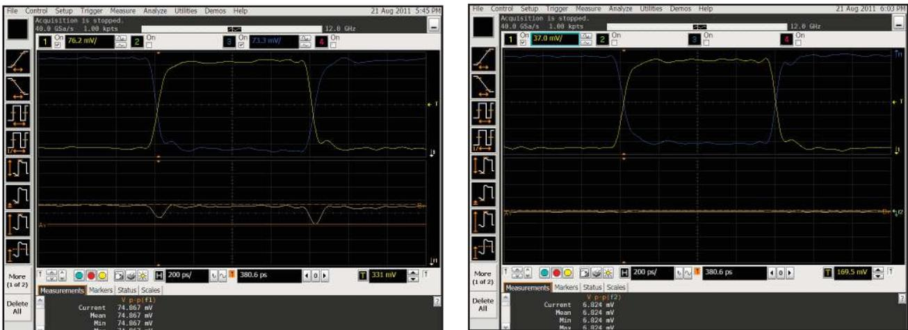
Figure 4. The left side screenshot shows probes with slightly different frequency responses when making common-mode voltage measurement. The result shows 75 mV, which is mainly caused by probes frequency response that are not exactly matched. On the right side, well-matched probes are used for the same measurement and the results show only 7 mV of common-mode voltage, which is the true performance of your design
