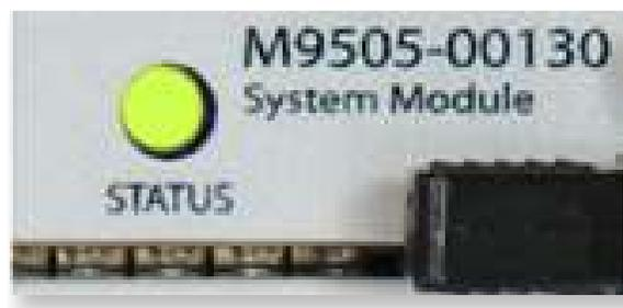
Figure 2. AXIe status light on ESM module must be green before powering-up controller.
