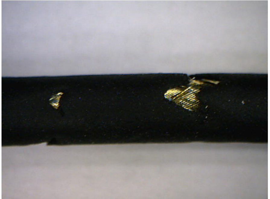
Figure 1: Regular probe cable damaged after environmental test at 120 °C.
