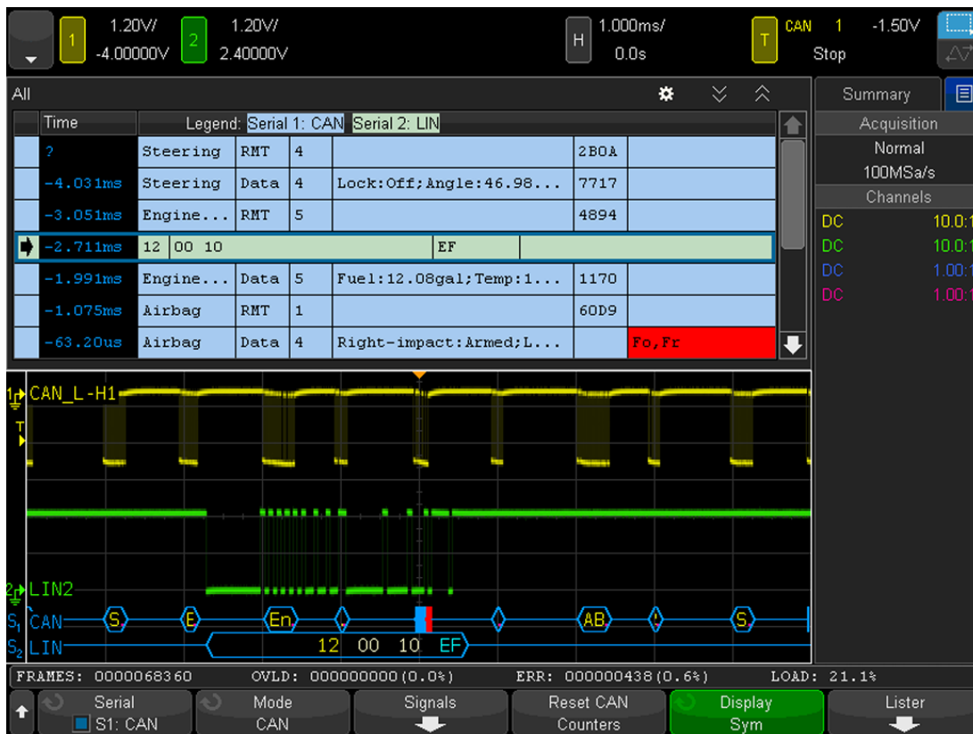
Figure 1(a). Decoding a LIN bus and CAN bus simultaneously using a Keysight InfiniVision X-Series oscilloscope
