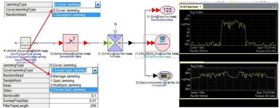
Figure 8. Common forms of jamming and counter-measures are selectable as a model parameter.
