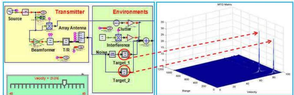
Figure 9. Multiple targets can be set up in the simulation framework, each with its own 3D position and velocity, in order to test the resolution of radar receiver algorithms and hardware prototypes.
