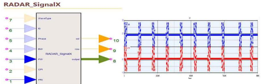
Figure 7. Dynamic pulse generation - Many of schematic parameters for radar pulse generation, such as repetition interval, carrier frequency, and phase, are externalized as live simulation pins using the "SignalX" component. This enables pulse characteristics to be encoded dynamically on each pulse, either from an external file, or from algorithms present in the simulation, which may be adapting to changing conditions.
