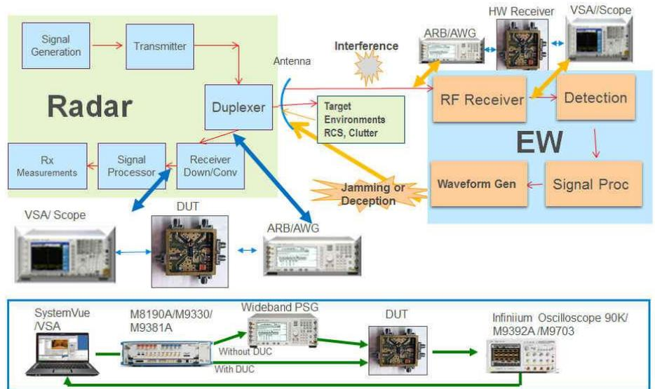
Figure 4. Waveforms at various locations in the simulation can be generated with live test equipment, or captured and brought into the simulation for further processing.
