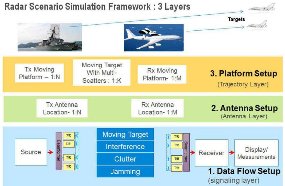
Figure 10. SystemVue offers additional layers for absolute position/velocity ("Platform") and beamforming/rotational direction ("Antenna"). This enables the 3D motion necessary for evaluating air/sea/sky radar platforms under realistic conditions.
