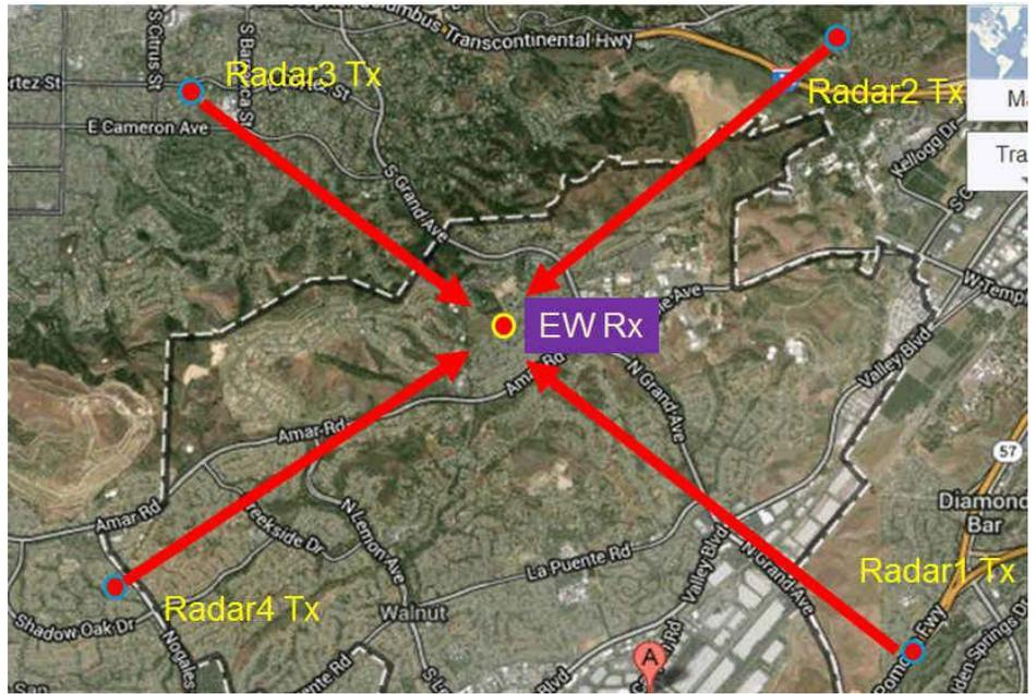
Figure 1. Shown here is an example of an EW receiver test environment, with several geographically dispersed emitters contributing to signal conditions at a centrally-located receiver. SystemVue helps make this modeling task easier, with lower NRE.
