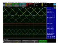
Figure 2. Visualize 4 dynamic power channels simultaneously
