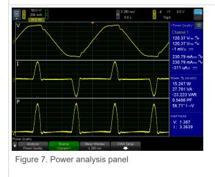
Press the [Analyze] key to view power quality measurements, shown in the blue Power Quality analysis panel. While displaying live power quality measurements, you can also view real-time voltage, current, and power waveforms
