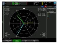
Figure 4. Phasor diagram for phase relationship analysis
