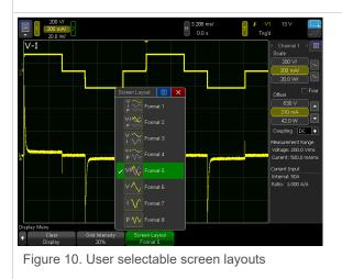
Choose from 8 different screen layouts of the voltage, current, and power waveforms. Here, the Keysight IntegraVision power analyzer displays an enlarged view of voltage and current on the same grid to highlight the time relationship between voltage and current.
