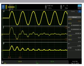
Use cursors to make common measurements, shown in the right-side panel. Here, the Keysight IntegraVision power analyzer displays in-rush current (middle current trace) and power (bottom power trace) following an AC line input voltage turn-on (top voltage trace). The cursors show a peak of 6.75 A during the first cycle.
