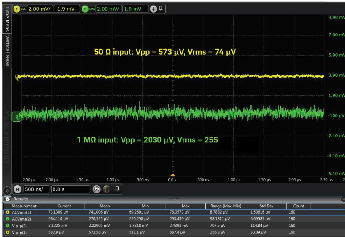
Figure 1. Baseline noise comparison of 50 \Omega and 1 M \Omega scope input of a Keysight Infiniium MXR054B
