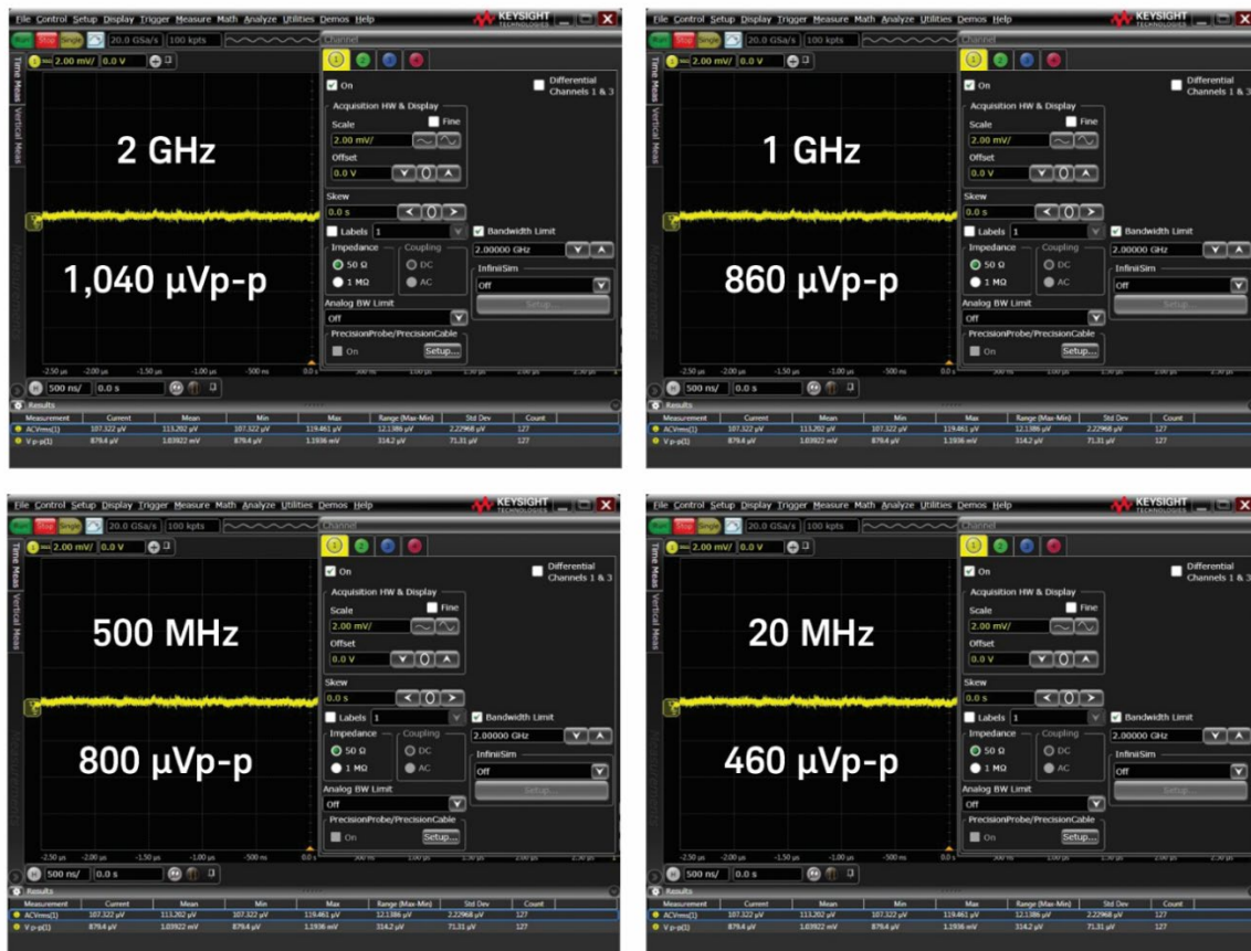
Figure 2. Baseline noise at various bandwidth limits with the Keysight N7020A power rail probe and MXR B-series oscilloscope
