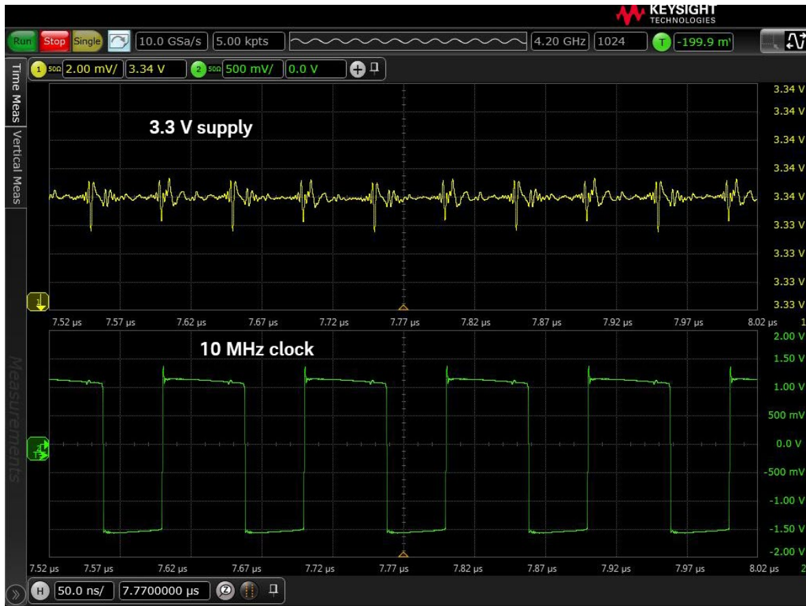
Figure 11. Triggering on the 10 MHz clock and enabling averaging removes all random noise and signals that are not coherent with the clock. The resulting view is of the noise on the supply related to the 10 MHz clock.
