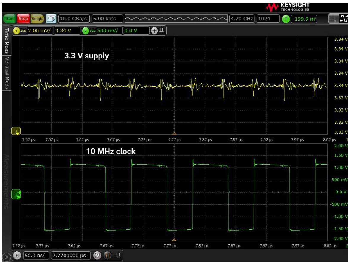
Figure 10. Measurement results of a 3.3 V supply and a 10 MHz clock in the target system. Using an FFT, we verify that the 10 MHz clock is creating noise on the 3.3 V supply.
