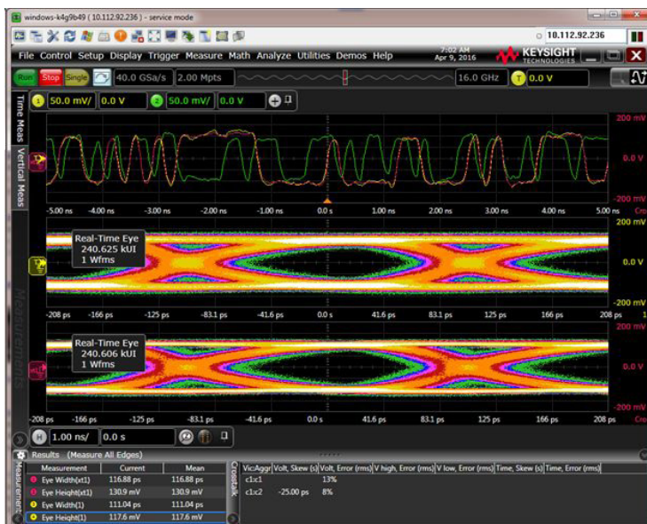
Figure 13. View eye width and height of victim signal with crosstalk and compare to signal without crosstalk.
