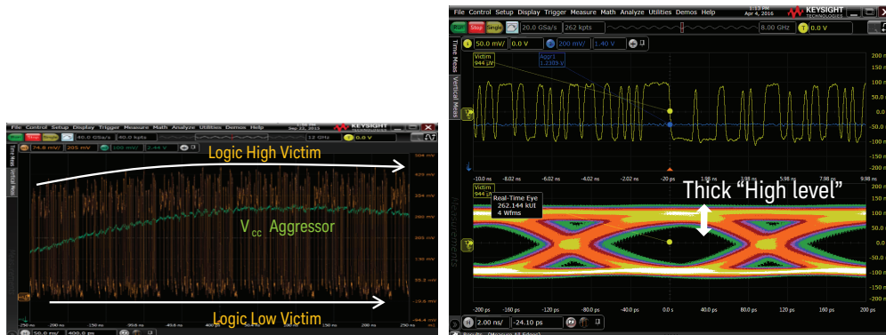
Figure 8. (Left image) Similar amplitude ramps of logic high and Vcc aggressor signals. (Right image) Thick high level of eye diagram caused by Vcc aggressor signal on logic high victim signal.
