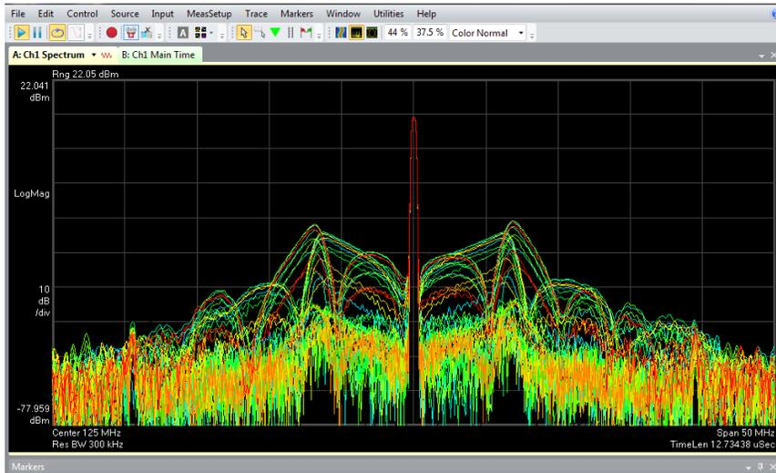
The PDN interrogation using the comb's search mode signal reveals a resonance at approximately 7.5MHz as seen in the spectrum sidebands around the clock fundamental frequency. Note the peaks are approximately -30dBc
