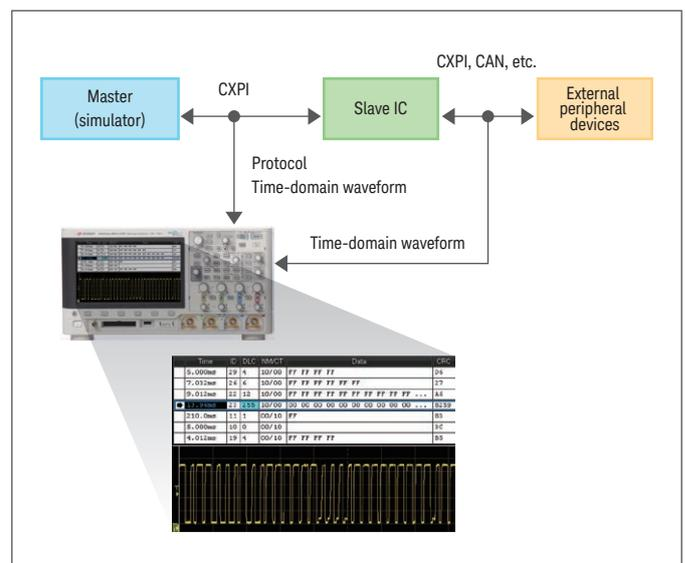
Figure 2. Design verification system for master-slave communication with a CXPI bus analyzer using the InfiniiVision 3000T X-series oscilloscope
