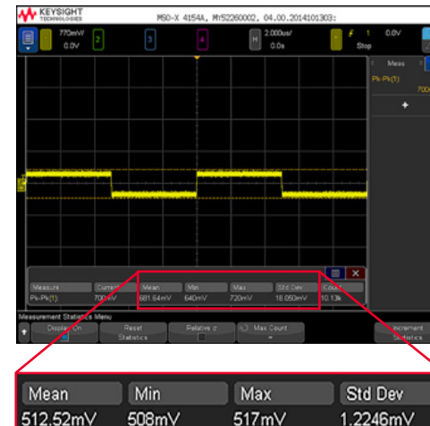
100 KHz clock signal
