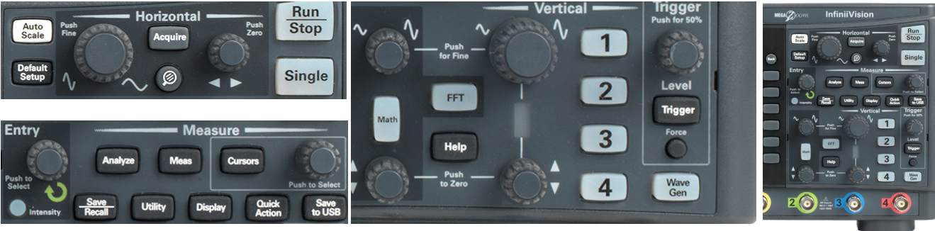
Figure 2. Oscilloscope front panels should include knobs for all key setup variables.
