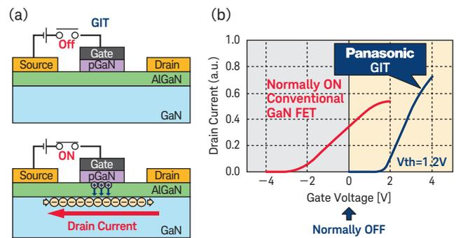
Figure 2 (a) shows the device structure. P-type GaN layer is used for the gate electrode to form a p-n junction. Figure 2 (b) shows the plot of the drain current vs the gate voltage. The GIT structure makes the device such that when its gate turns on, holes are injected into the channel.
