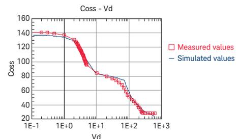
The graph shows the results from analysis using models named ASM for GaN power transistors, and S-parameter models for evaluation boards using an RF/microwave circuit simulator named ADS. Note that the measured values and simulated values match very well. Ciss (input capacitance) and Crss (reverse transfer capacitance) also show a similar correlation.
