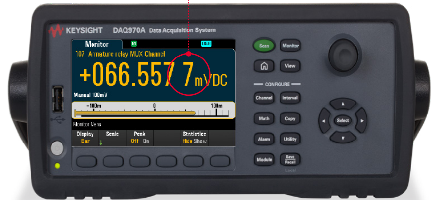
Figure 15. Lowest voltage resolution measured by this DAQ system
