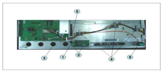
**Step 1.** Replace the prove power board or switch board by inverse procedure of removal.
