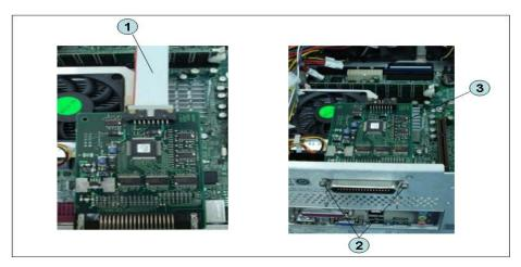
**Step 1.** Replace the handler I/O board by inverse procedure of removal.
