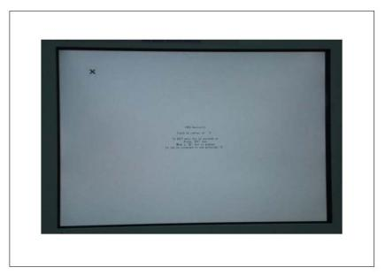
**Step 5.** Touch the x mark on the upper left with your finger. The mark x appears also on the lower left, upper right, and lower right. Touch the x marks in that order with your finger.
