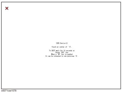
**Step 5.** Touch the x mark on the upper left with your finger. The mark x appears also on the upper right, lower left, and lower right. Touch the x marks in that order with your finger.
