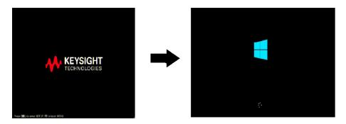
If you encounter the following problems, try to reinstall the operating system before replacing the Hard Disk Drive.
