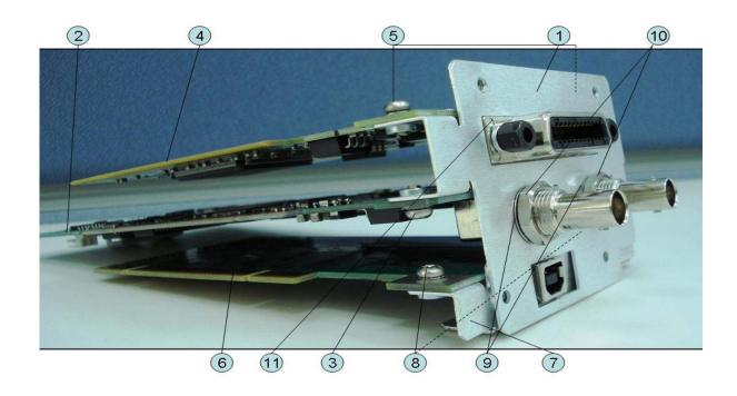
Table 5-40 PCI DSP Card, GPIB Card AND USB Card Assembly (Serial number prefix MY461 or SG461)
