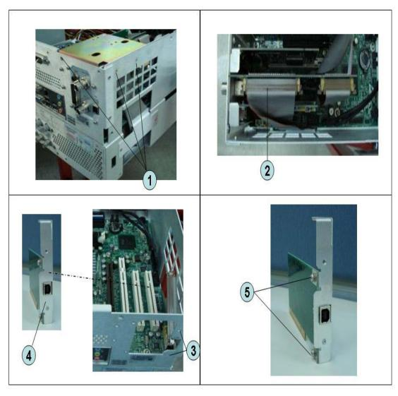
**Step 1.** Replace the USB (USBTMC) interface card by inverse procedure of removal.
