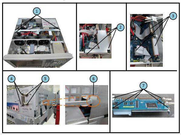
**Step 1.** Replace the PCI-E DSP card and GPIB cable by inverse procedure of removal.
