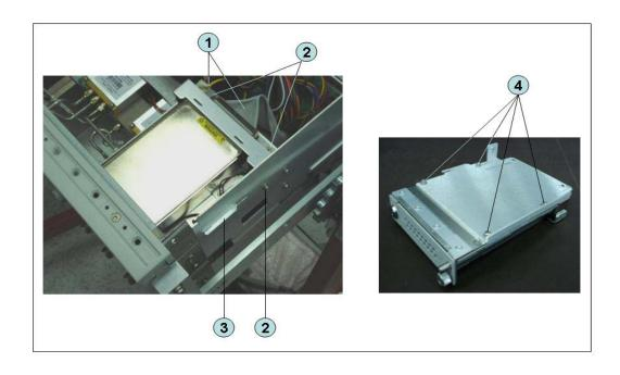
Figure 6-7 Removable Hard Disk Assembly Replacement Option 017 (Serial number prefix MY462/MY463 or SG462/SG463)
