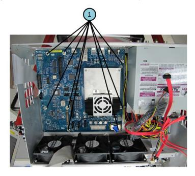
**Step 1.** Replace the digital motherboard by inverse procedure of removal.
