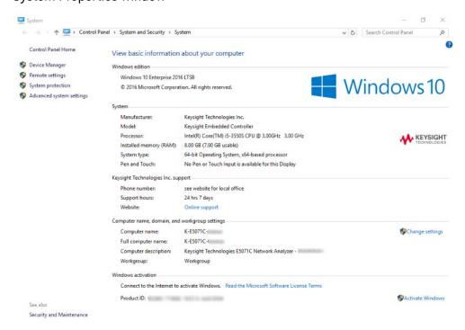
**Step 7.** Verify that the amount of RAM installed is correct. Table 4-17 shows the amount of RAM memory installed depending on the Digital Motherboard. If the amount of RAM installed is not correct, the CPU Mother Board Assembly is faulty.
