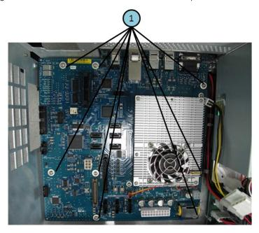
Figure 6-21 Digital Motherboard Removal (Serial number prefix MY463 or SG463)
