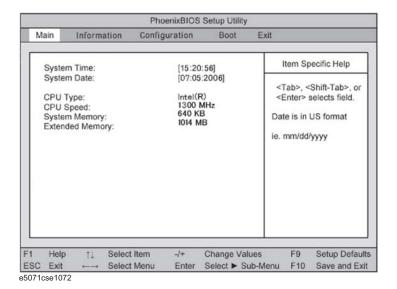
Step 6. Choose "Exit" using — keys and select "Load Setup Defaults" using telest. Keys. The dialog box "Setup Confirmation" prompts you to select Y (Yes) or N (No). Press Y and Enter to load the manufacture Setup Defaults into the BIOS ROM. As a result, almost all of the BIOS options are automatically configured to the optimal settings for the E5071C.
