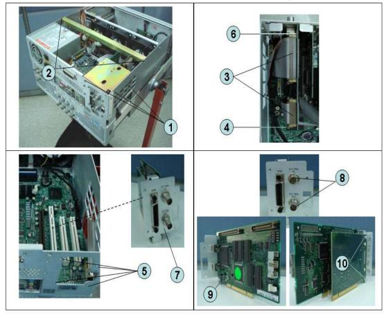
Step 1. Replace the PCI DSP card and GPIB card by inverse procedure of removal.
