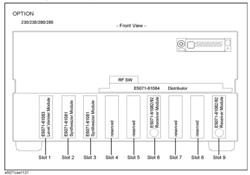
Slot 2: Synthesizer Module for Source
