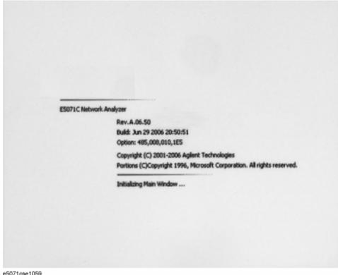
If the display whited out, entirely blued or appeared with a dialog box, a mass storage problem is suspected. Try to perform the mass storage recovery procedure.
