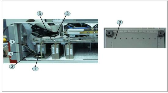
**Step 1.** Replace the doubler module by inverse procedure of removal.
