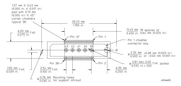
Board pad details of MICTOR connector and support shroud
