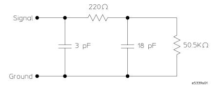
Equivalent probe load
