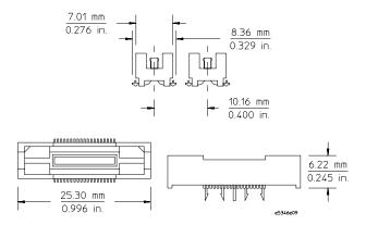
38-pin MICTOR connector dimensions
