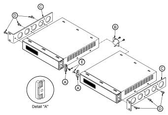
4. Using Pozidriv screwdriver, attach Rack Ear-Full Rack (C) to each E5810/E5818 with six M4x10 Panhead Screws (D).
