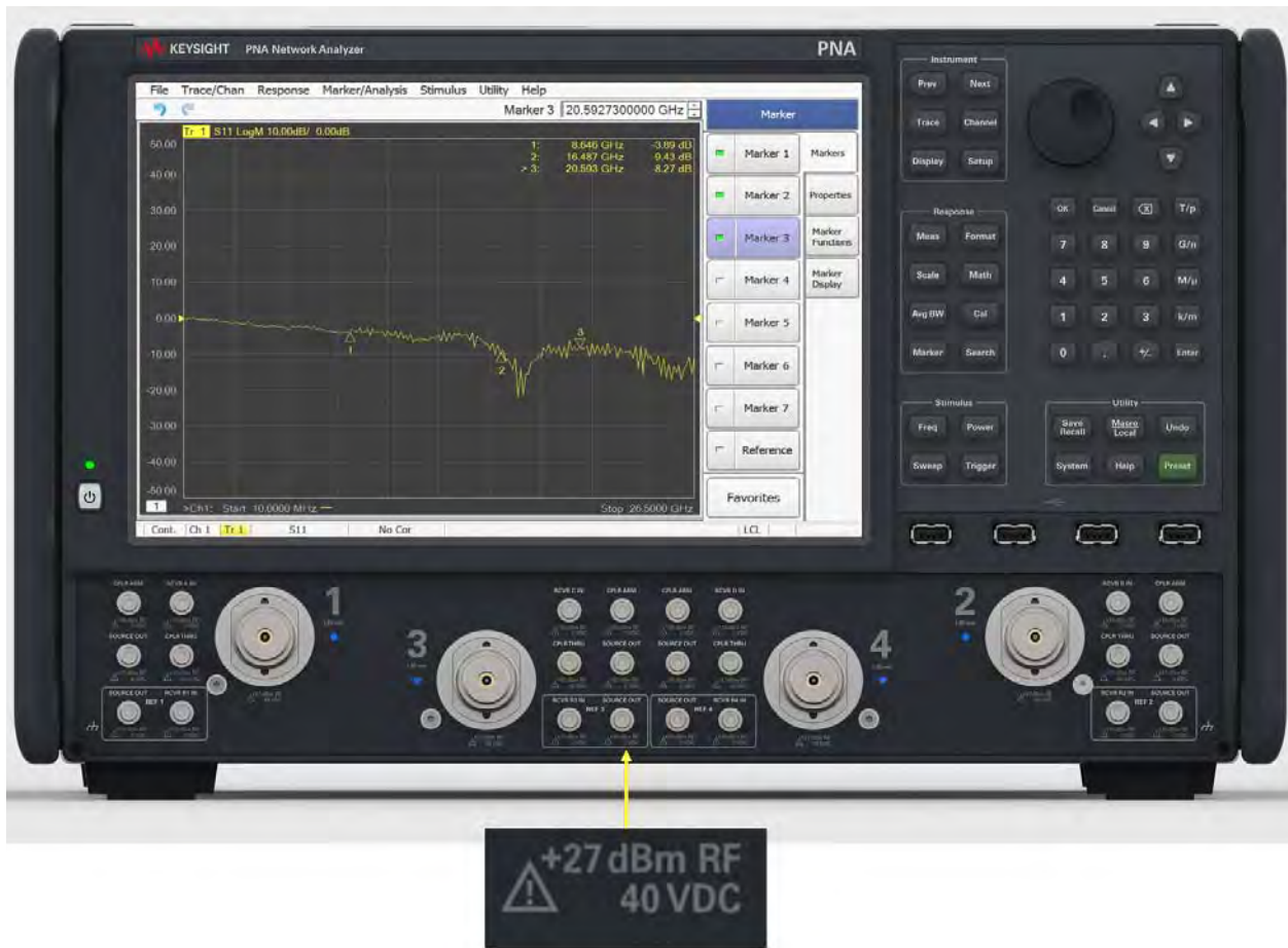
Figure 2 Example Label Showing Damage Level for Each Port and Connector
