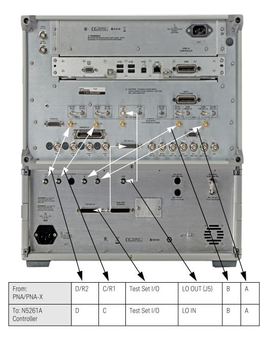
Figure 1-16 N5262A Rear Panel Configuration B
