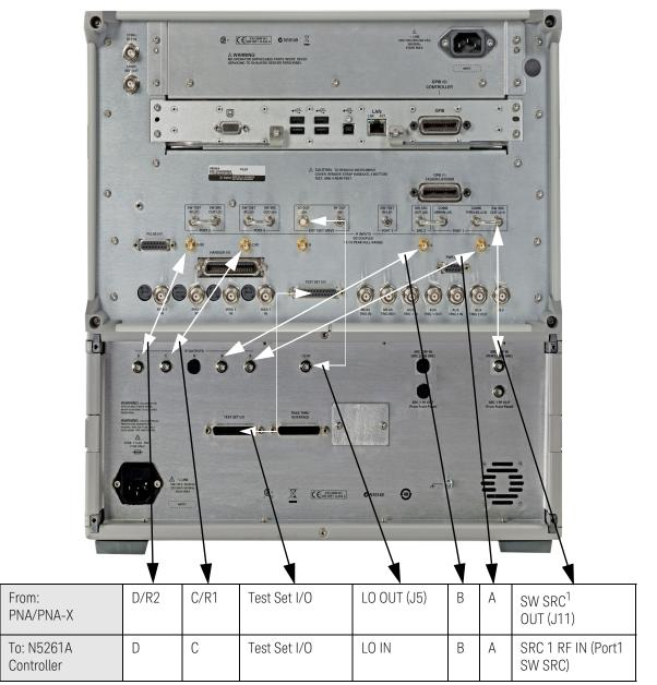
1. Install the adapter (N4903-61250) on the N5224/25A/B or N5244/45A/B SW SRC OUT (J11).
