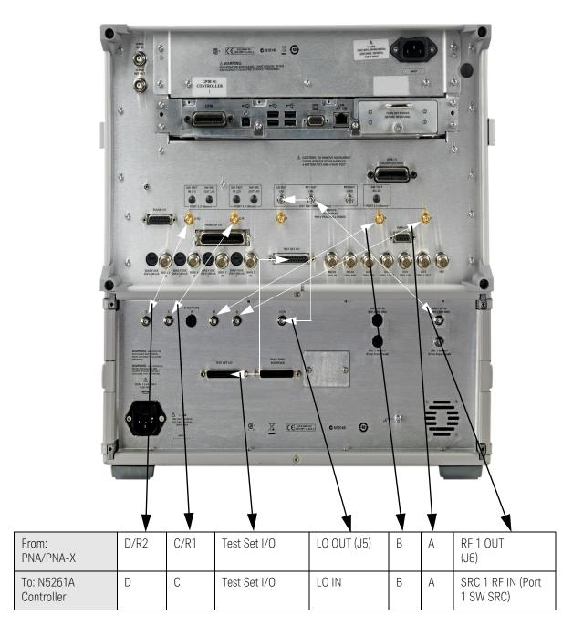
Figure 1-20 N5262A Rear Panel Configuration F
