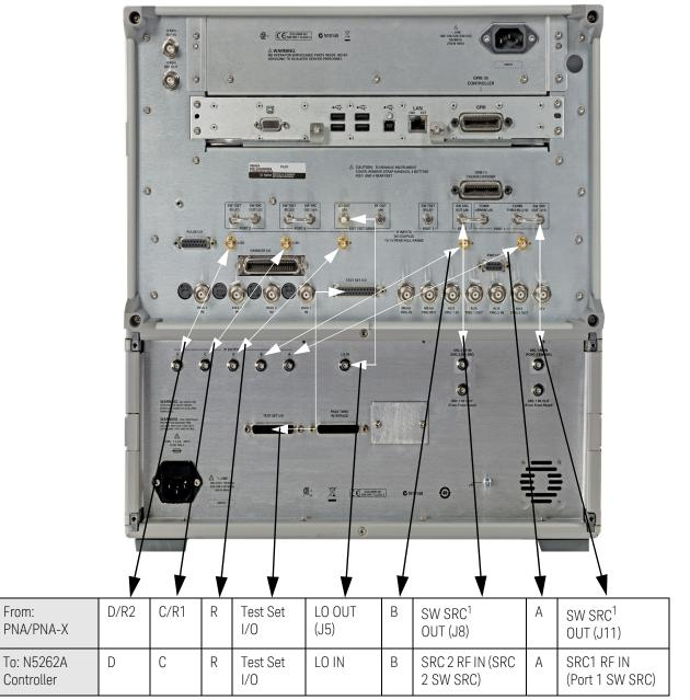
1. Install the adapters (N4903-61250) on the N5224/25A/B or N5244/45A/B SW SRC OUT (J8 and J11).
