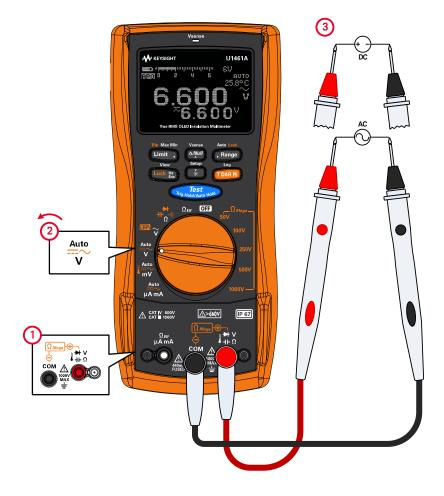
Figure 2-11 AC or DC voltage measurement example
