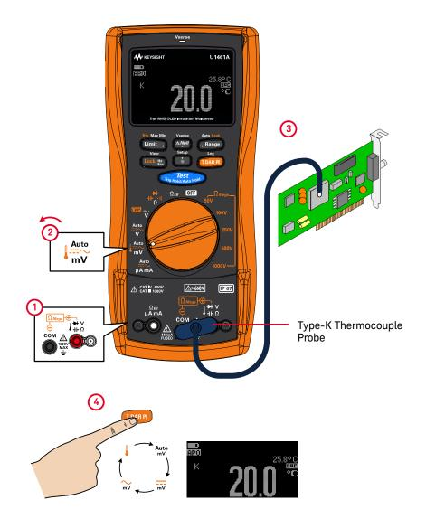
Figure 2-22 Surface temperature measurement example
