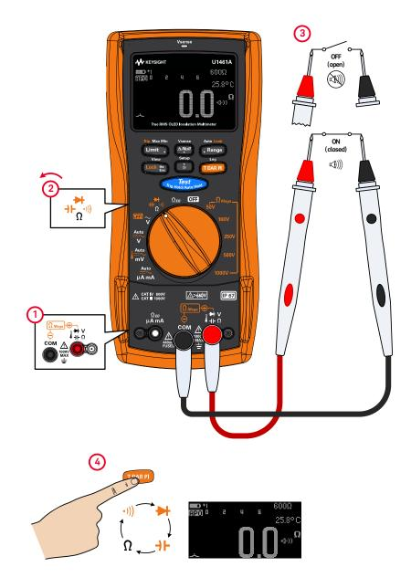
Figure 2-17 Continuity test example
