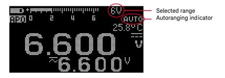
Pressing changes the tester range (and disables auto-ranging). Each additional presses of range (in manual ranging) sets the tester to the next higher
