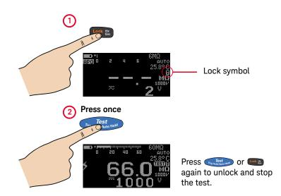
By default, the tester will reset the locked status when the test is stopped by pressing for the lock once feature" on page 149 to disable this feature.
