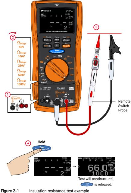
Insulation resistance test example
