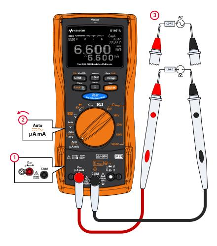
Figure 2-14 AC or DC current measurement example
