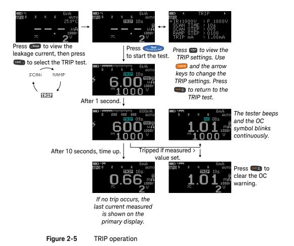
Set up your tester as shown in Figure 2–1, and follow the steps shown in Figure 2–5.
