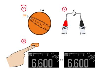
Figure 2-12 AC voltage with LPF measurement example
