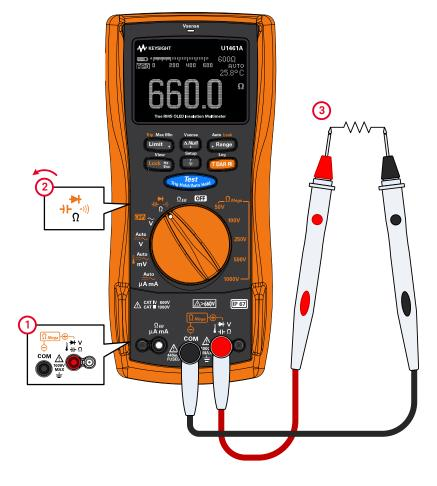
Figure 2-16 Resistance measurement example
