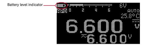
Replace the batteries as soon as possible when the low battery indicator (  $\boxplus \leftrightarrow$  time) flashes.
