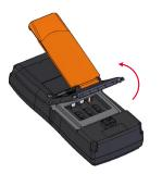
**3** Lift and remove the battery cover as shown on the left.
