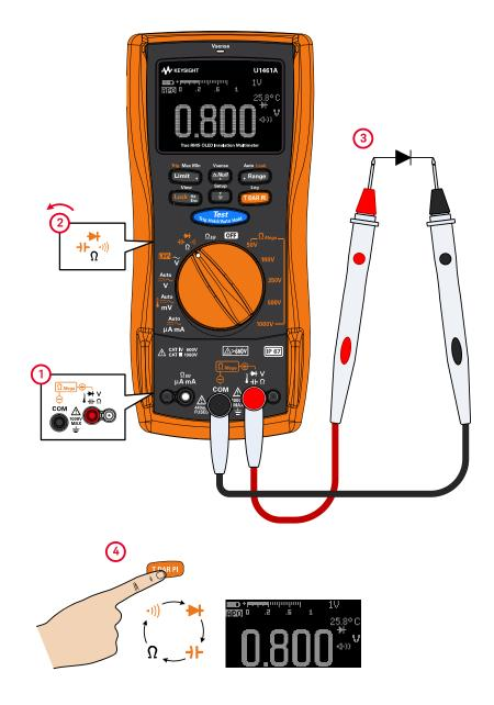
Figure 2-18 Forward-bias diode test example
