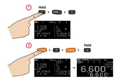
Figure 2-13 Enabling the low-pass filter
