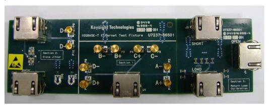
Figure 1 Complete U7237A 10GBASE-T Transmitter Test Fixture Board
