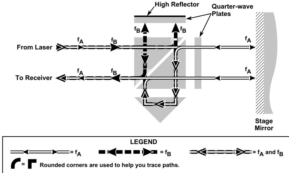
**Figure 15-3. Agilent 10706B High Stability Plane Mirror Interferometer Beam Paths**
