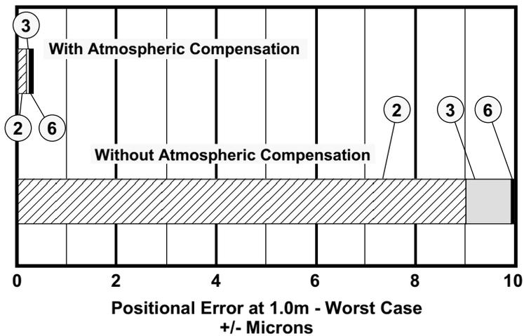
**Figure 15-12. Worst-case System Repeatability with and without Atmospheric Compensation for the CMM example**
