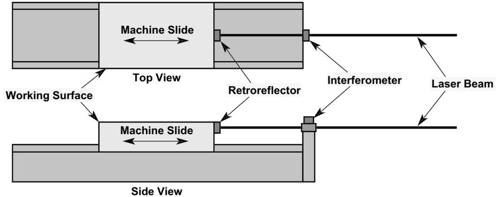
**Figure 15-22. Positioning of measurement axis to minimize Abbé error**
