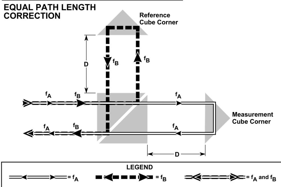
Figure 15-21. Equal path length correction
