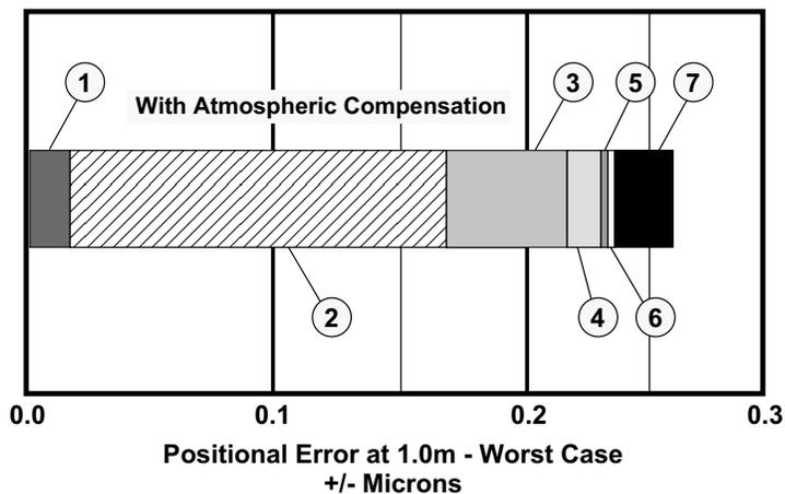
**Figure 15-11. Worst-case System Accuracy with Atmospheric Compensation for the CMM example**
