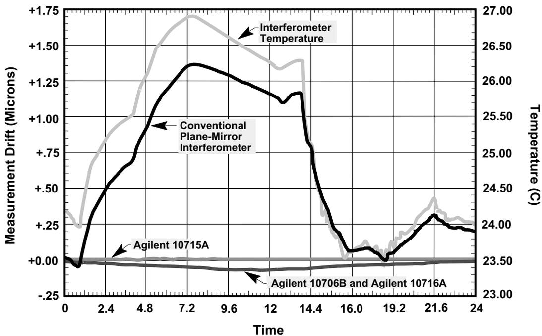
**Figure 15-4. Comparison of optics thermal drift between Interferometers**
