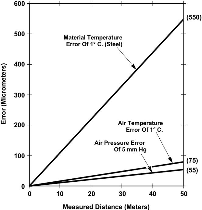
Figure 15-19. Relative effect of errors in atmospheric and material temperature
