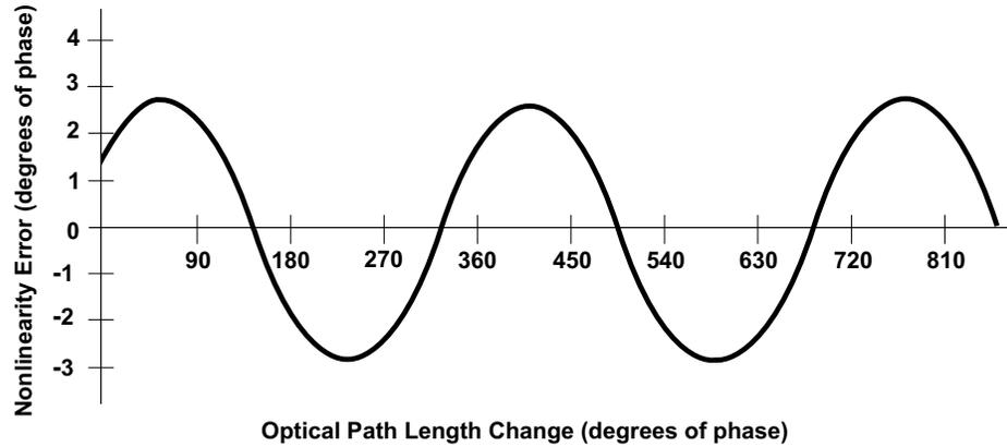
**Figure 15-1. Worst-case error resulting from imperfect separation of two beam components**
