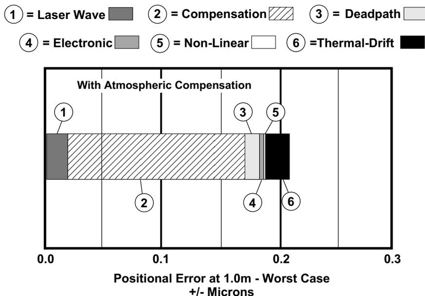
**Figure 15-13. Worst-case System Repeatability with Atmospheric Compensation for the CMM example**
