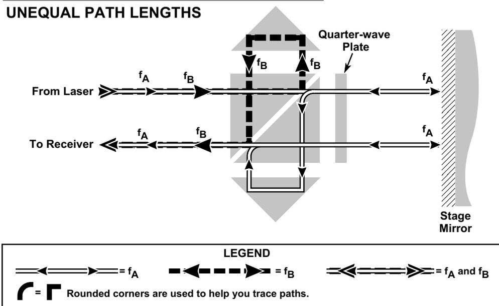
**Figure 15-2. Conventional plane mirror interferometer with unequal path lengths that result in optics thermal drift**
