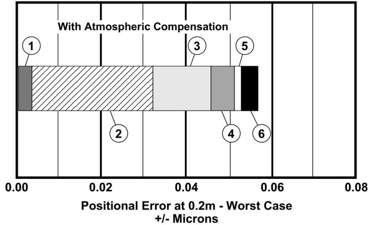
**Figure 15-18. Worst-case System Long-term Repeatability with Atmospheric Compensation for the Wafer Stepper example**
