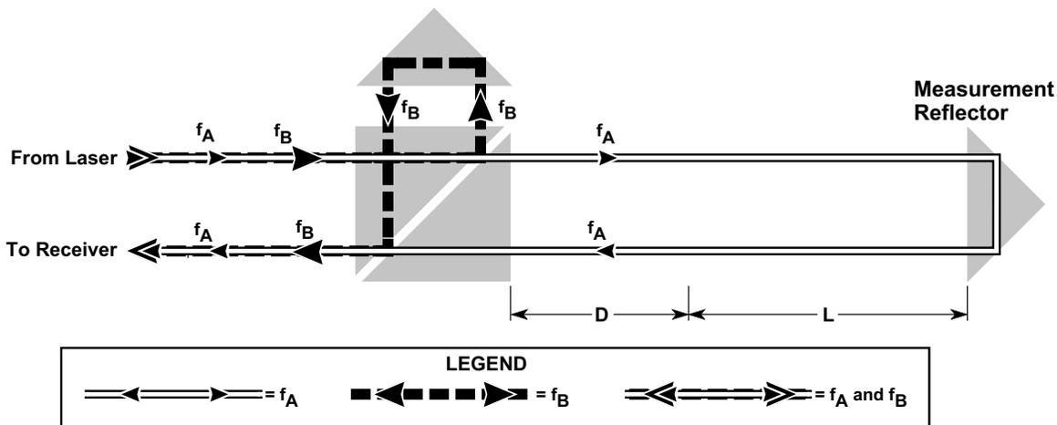
**Figure 15-5. Deadpath caused by unequal lengths from initial point**
