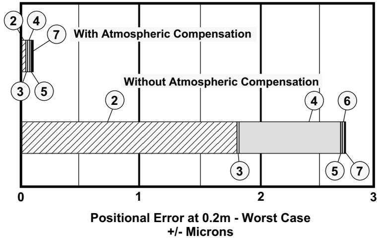
**Figure 15-15. Worst-case System Accuracy with and without Atmospheric Compensation for the Wafer Stepper example**
