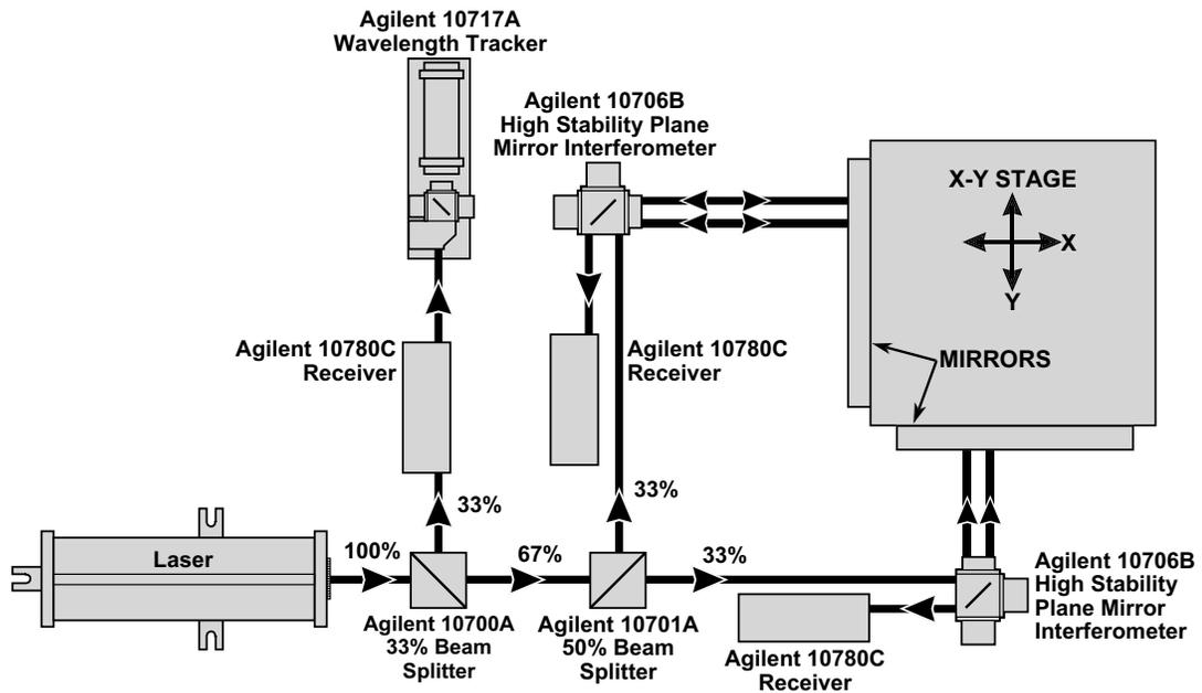
**Figure 15-14. Laser System Configuration for an Integrated Circuit Wafer Stepper**
