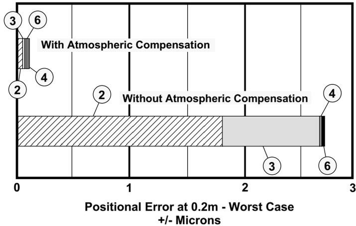
**Figure 15-17. Worst-case System Long-term Repeatability with and without Atmospheric Compensation for the Wafer Stepper example**
