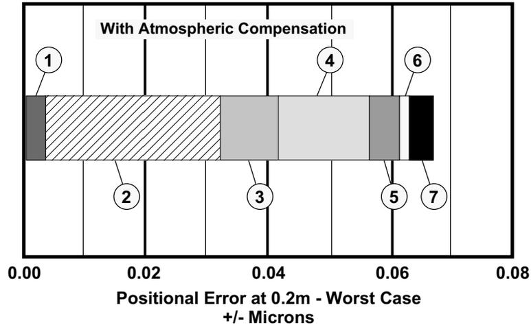
**Figure 15-16. Worst-case System Accuracy with Atmospheric Compensation for the Wafer Stepper example**
