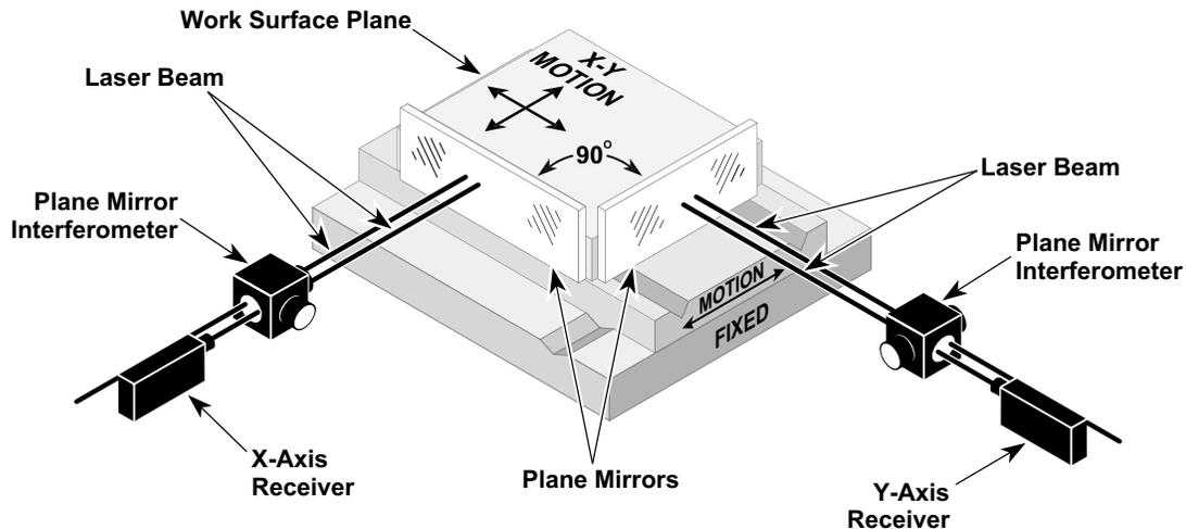
**Figure 15-23. X-Y Stage measurement with Agilent 10706A Plane Mirror Interferometer**
