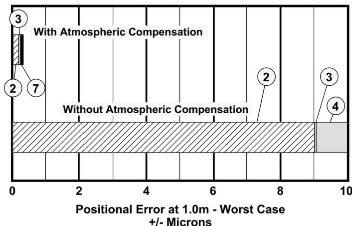
**Figure 15-10. Worst-case System Accuracy with and without Atmospheric Compensation for the CMM example**
