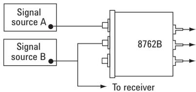
Figure 4. Multi-source switching
