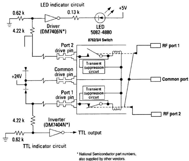
Figure 7. TTL and LED remote indicator circuits
