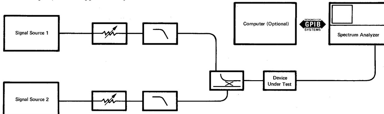
Figure 1. Test Setup for Third Order IMD Measurements
