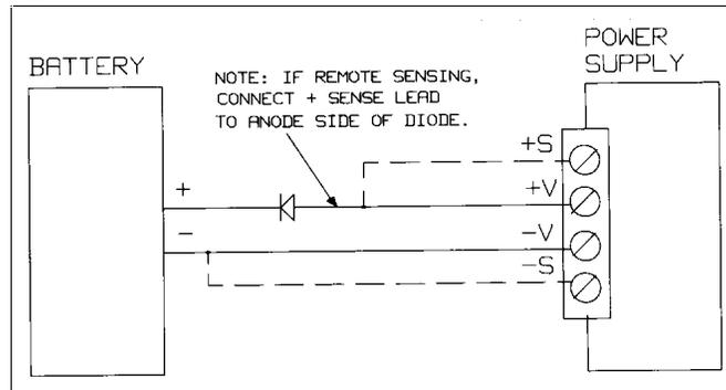
**Figure 4-10. Recommended Protection Circuit for Battery Charging**
