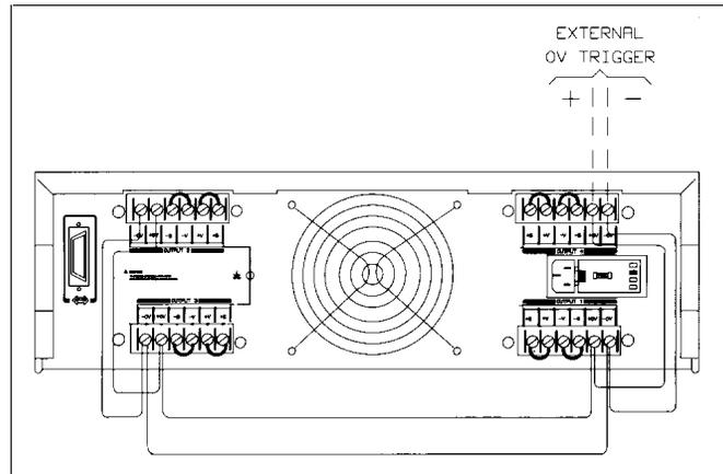
**Figure 4-7. Overvoltage Connections**
