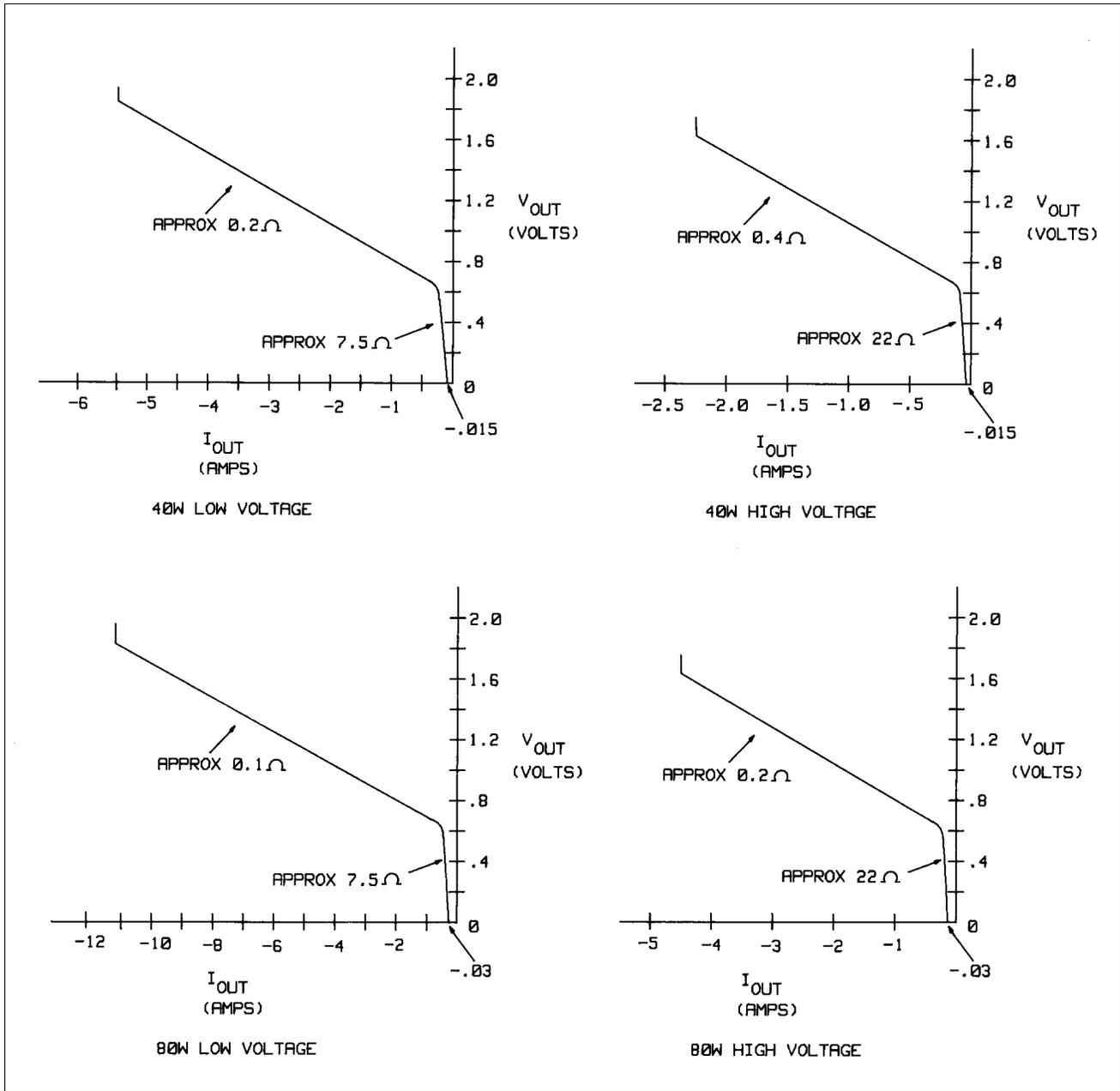
Figure 4-3 Typical Downprogramming Characteristic Below 2.0 V
