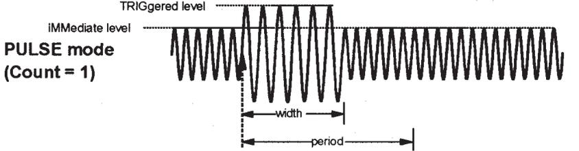
At trigger, the triggered level is active during the pulse width portion of the pulse waveform.
