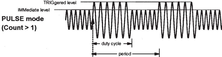
At trigger, the triggered level is active during the duty cycle portion of the pulse waveform.
