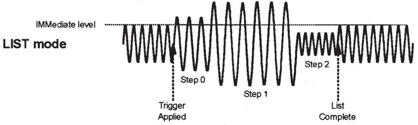
At trigger, the list starts. When list completes, the output returns to immediate level. Steps 0, 1, and 2 can be set to repeat from 1 to infinity upon receipt of trigger.
