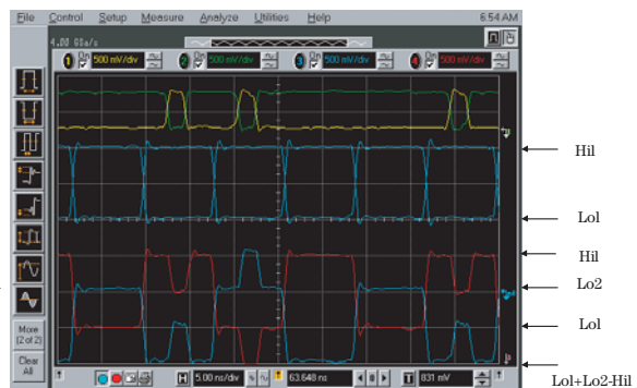
Fig 9b : Analog channel Add Agilent E4838A Frontend
