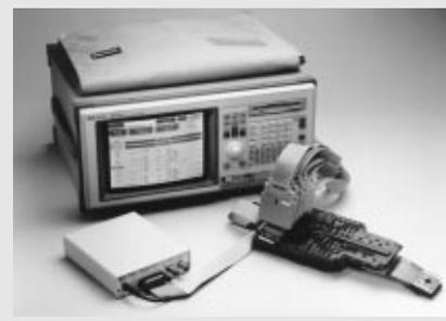
However, firmware engineers often use real-time trace analysis and sometimes need very deep trace history. To satisfy their requirements at low cost, they could choose the HP 1671D portable logic analyzer, for example, which supports up to a 100 MHz state and 1 M trace depth. (Figure 3)
