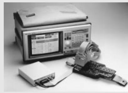
However, firmware engineers often use real-time trace analysis and sometimes need very deep trace history. To satisfy their requirements at low cost, they could choose the HP 1671D portable logic analyzer, for example, which supports up to a 100 MHz state and 1 M trace depth. (Figure 3)
