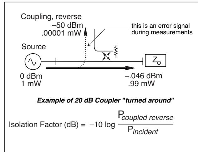
Figure 4. Directional Coupler Isolation (Reverse Coupling Factor)
