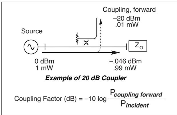
Figure 3. Forward Coupling Factor
