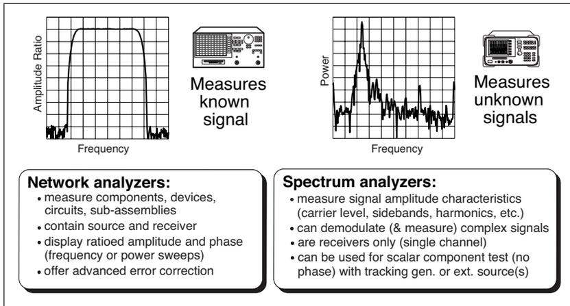
Figure 1. Differences between Network and Spectrum Analyzers
