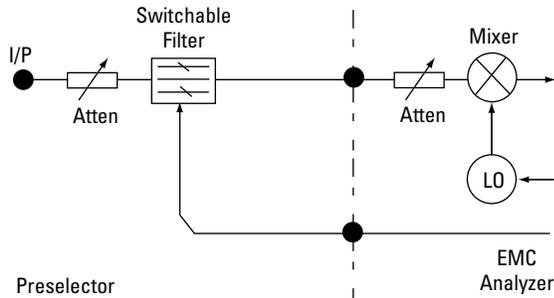
The Agilent Technologies 11960A EMC preselector is a series of switched band pass filters designed to reduce the bandwidth of the energy present at the first mixer of the EMC analyzer.
