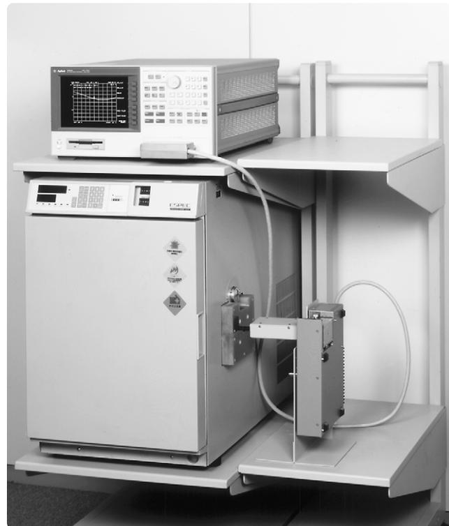
Figure 8. Configuring a system using a Tabai Espec chamber
