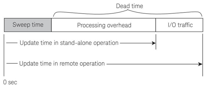
Figure 1. The components of measurement update time.
